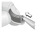
**Important:** Do not force the battery door beyond its fully opened position. Excessive force can deform the battery door, which will reduce its tamper resistant effectiveness.
