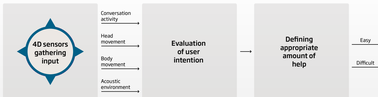
Figure 3. The process of the 4D Sensor technology: The 4D sensors gather input in the four dimensions, the input is evaluated to interpret the user intention and combined into a single set of parameters which define the appropriate amount of help for the remaining features in MSI 3.0 to act upon.
