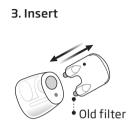
Insert the new wax filter using the other pin. Remove the tool, and throw it out.
