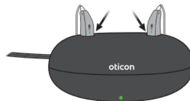
The hearing aid LED lights turn ON when the hearing aids are correctly placed in the charger.
