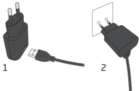
1. Insert the USB plug into the power plug.
