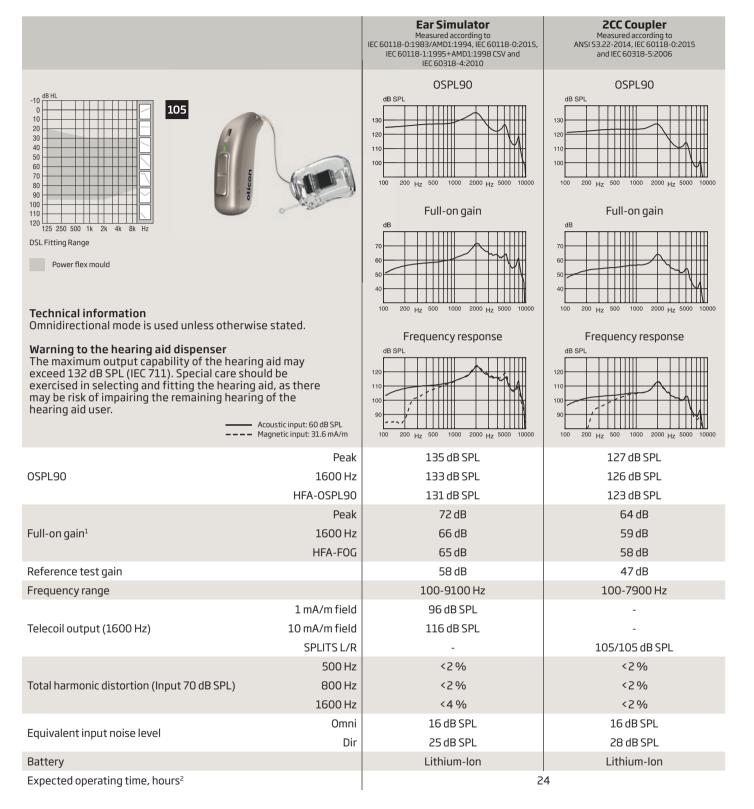
1) Measured with the gain control of the hearing aids set to their full-on position minus 20 dB and with an input SPL of 70 dB. This is to obtain a gain response equal to the full-on gain response from e.g. IEC 60118-0:1983+A1:1994 but without influence of feedback.
