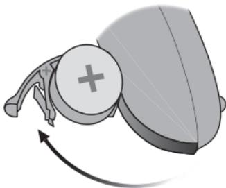
Open the battery drawer fully. Remove the battery.
