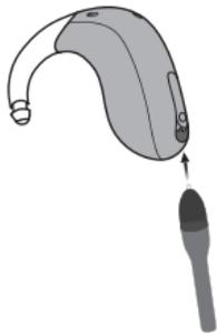
Insert tool into hole at the bottom of the push-button.
