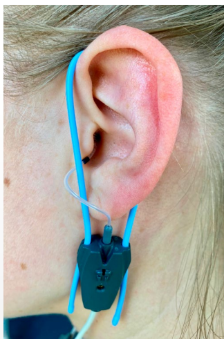
Figure 1. Probe tube passed around the lanyard. Note the black marker ring.
