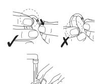
Make sure the ear mould and tubing are completely dry before they are reconnected to the hearing instrument. Be careful that left ear mould and tubing are connected to the hearing instrument with left ear marking and vice versa for the right ear instrument.
