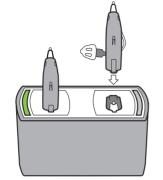
Plug the USB into the charger, then plug the adapter into the wall. Once powered, the charger LED will shortly blink green. Place your hearing aids into the charger dock. You will see a green light blinking when the hearing aids start charging.
