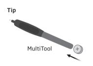
The MultiTool can be used to change the battery. Use the magnetic end to remove and insert batteries.
