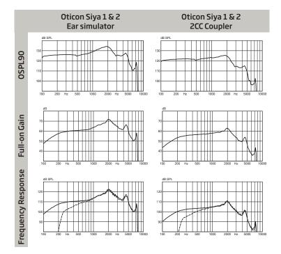
Acoustic input: 60 dB SPL --- Magnetic input: 31.6 mA/m
