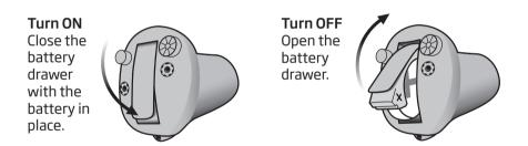
**Note:** Open the battery door fully to make sure the hearing aid does not drain the battery fully and to allow air to circulate whenever you are not using your hearing instrument, especially at night or for longer periods of time.
