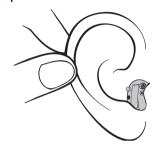
Gently pull your ear outwards and push the hearing aid into the ear canal, twisting slightly if necessary. Follow the natural contour of the ear canal. Push the hearing aid to make sure it fits comfortably in the ear.
